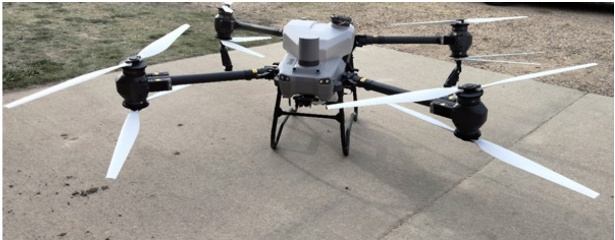
Figure 1. Spray drone with white propellers made out of nylon carbon fiber filament and equipped with a dual atomizing spraying system (spray tank, centrifugal sprinklers, and magnetic drive impeller pumps), phased array radar system, and binocular vision system. Photo by Jeremie Kouame, Kansas State Research Extension
