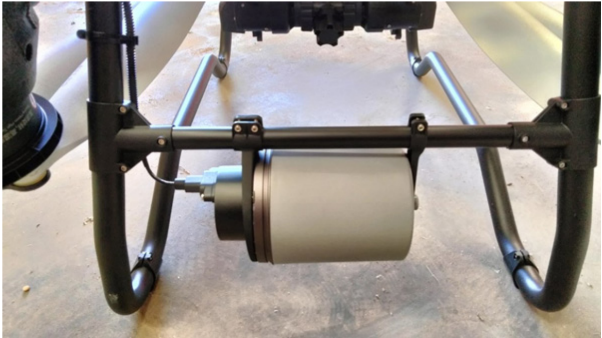
Figure 2. Rear phased array radar system for terrain follow. Photo by Jeremie Kouame, Kansas State Research and Extension.
